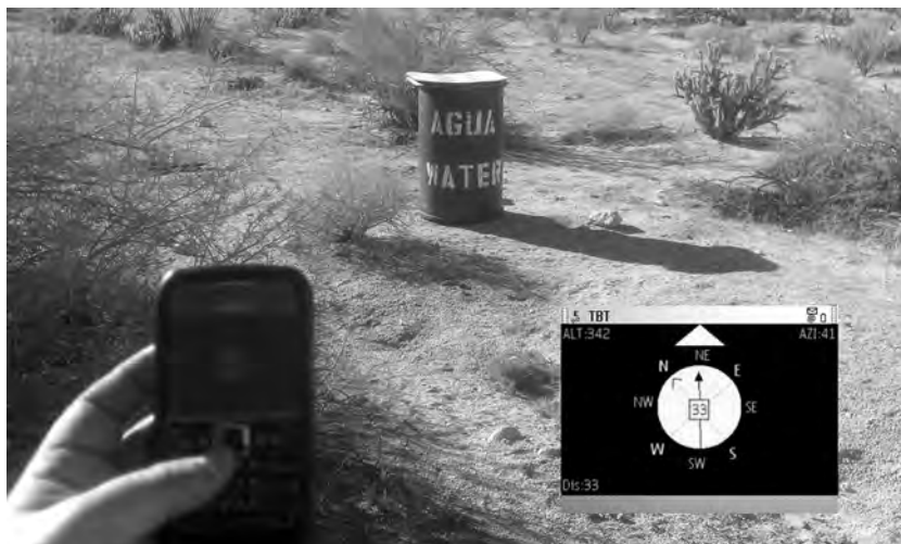
Figure 36 Electronic Disturbance Theater (EDT)/b.a.n.g. lab: Transborder Immigrant Tool, a cell phone hack distributed along the US–Mexico border in 2009 to assist individuals crossing the US–Mexico border using a built-in GPS app to locate water left by volunteer groups and medical help centers
